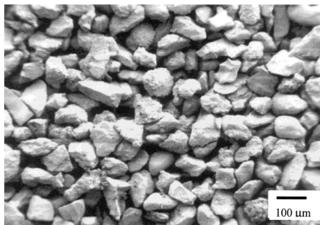
Figure 18. SEM image of a Chinese dust sample with grain size, d , of 54 \mu\text{m} < d < 85 \mu\text{m} . The image is of a sample used for Knudsen cell reactor experiments. (Reproduced with permission from Phys. Chem. Chem. Phys. 3, pp 2474–2482; F. Hanisch and J. N. Crowley. Copyright 2001 PCCP Owner Societies.)
